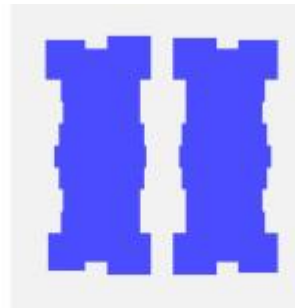
(b) Manhattan patterns with edge-based OPC
